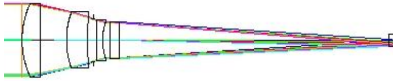
Figure 4. The optical layout of the metrology camera.
